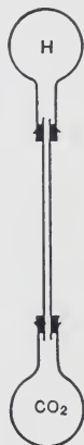
FIG. 25.— Appa- ratus to show Diffu- sion of Carbon Dioxide and Hy- drogen.
